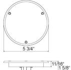
10 Surface Mount Diodes (SMD) Epoxy filled base Meets DOT FMVSS 108 requirements when installed as a pair Includes reflex reflector on mounting flange Available in flange mount style Requires industry standard 2-Prong plug
